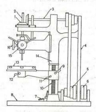
Figure Upright pillar drilling machine
