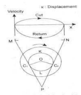
Figure 7.4 Principle of quick return mechanism
