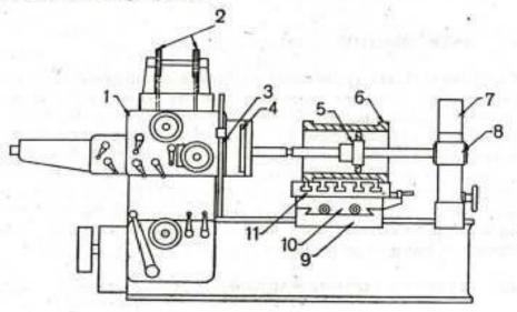
**Figure** Horizontal boring machine
