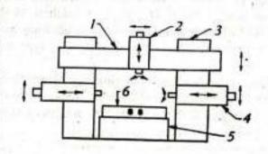
Figure Multiple head type horizontal boring machine 1. Crossrail, 2,4. Headstocks, 3. Column,
