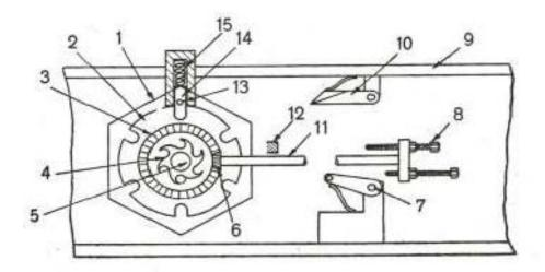
Figure 4.5 Turret indexing mechanism
