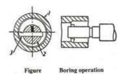
The work is revoluted in a chuck or a face plate and the tool which is flitted to the tool post is fed in to the work. One piece forged tool is used for boring small hole, whereas a boring bar with a tool bit attached to it is suitable for machining a large hole the doc is giver by the cross slide screw and the fade is feeder by the longitudinal travel of the carriage.
