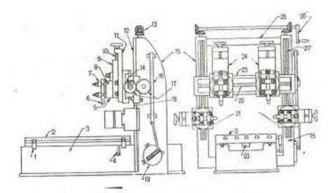
Figure 8.1 Standard double housing planer
