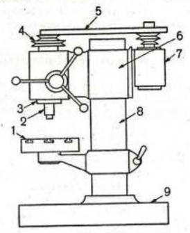
Sensitive drilling machine Figure 1. Table, 2. Vertical drill spindle, 3. Sleeve, 4. Cone pulley, 5. V-belt, 6. Head, 7. Driving motor, 8. Venical column, 9. Base.
