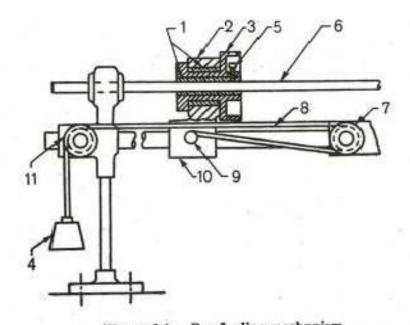
Chuck bush, 2. Sliding bracket body, 3. Bar chuck, 4. Weight, 5. Bar chuck set screw, 6. Bar, 7, 11, Pylley, 8. Chain, 9. Pin on the sliding bracket, 10. Sliding
