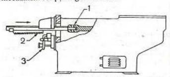
Figure Horizontal braoching machine 1. Pulling head, 2. Braoch, 3. Work fixture.
