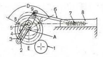
Figure Whitworth quick return mechanism
