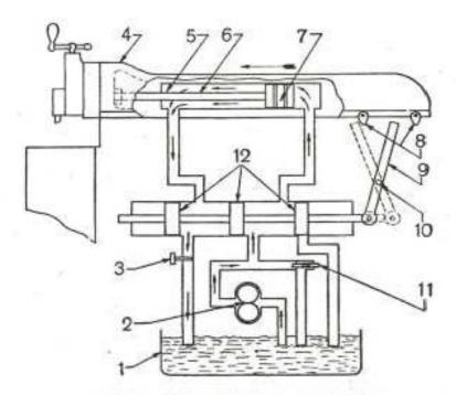
Figure 7.9 Hydraulic shaper mechanism
