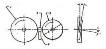
1. Grinding wheel, 2. Work, 3. Regulating wheel, 4. Work-rest.
