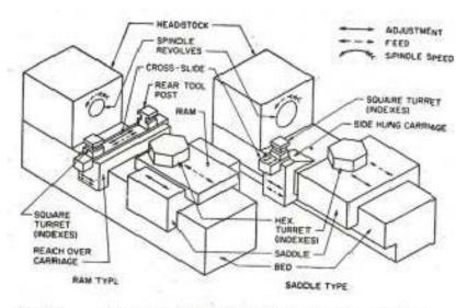
Figure Ram type (capstan) and saddle type (turret) lathes (Reproduced from Doyle et al)
