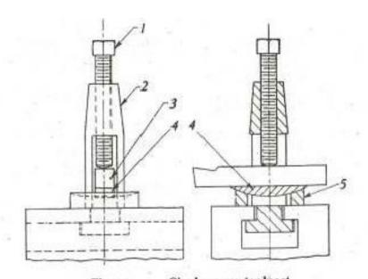
Figure Single screw toolpost
