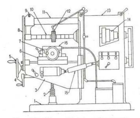
Figure 11.1 Column and knee type milling machine
