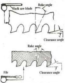
Figure Rake and clearance angles on back saw blade and file
