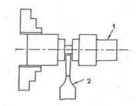
Figure 3.69 Parting off operation 1, Work, 2, Parting off tool.
