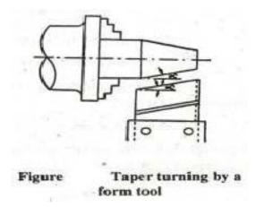
Abroad nose tool having straight cutting edge is set on to the work at half taper angle, and is feed straight into the work to generate a tapered surface. The half angle of taper will correspond to (90-SCEA) of the tool. The work is held in a chuck or clamped on a face plate.
