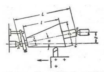
Figure Taper angle by setover method
