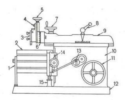
Figure 7.1 Parts of a standard shaper
