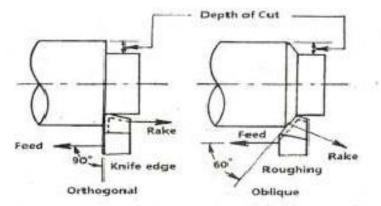
Figure Orthogonal and oblique cutting
