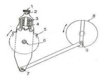
Figure 7.10 Automatic feed mechanism of a shaper
