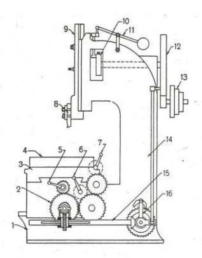
Figure 9.1 Slotting machine
