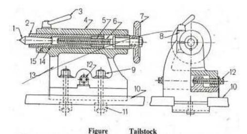
Dead centre, 2. Spindle, 3. Spindle clamp, 4. Barrel, 5. Bush, 6. Square threaded screw, 7. Hand wheel, 8. Split lug, 9, Tailstock clamping bolt, 10. Lathe bedways, 11. Clamping plate, 12. Sctover screw, 13. Body, 14. Keyway, 15. Key.
